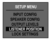
The Listener Position menu is used for setting the surround and center delays and calibrating the Panorama effect.
